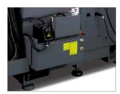
Oil cooler fitted as standard for rotary tools
